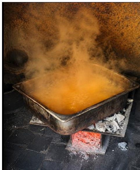
Fig 3: An acid solution containing dissolved gold is brought to a vigorous boil over an open charcoal fire, a step that drives off excess acid and concentrates the gold-bearing liquor. (Researchers Fieldwork, 2026)
