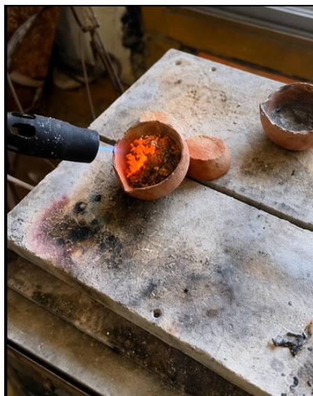
Fig 2: A handheld torch is used to burn mercury out of an amalgam held in a small clay crucible, producing the visible orange glow of the reaction and releasing mercury vapour into the open air. (Researchers Fieldwork, 2026)
