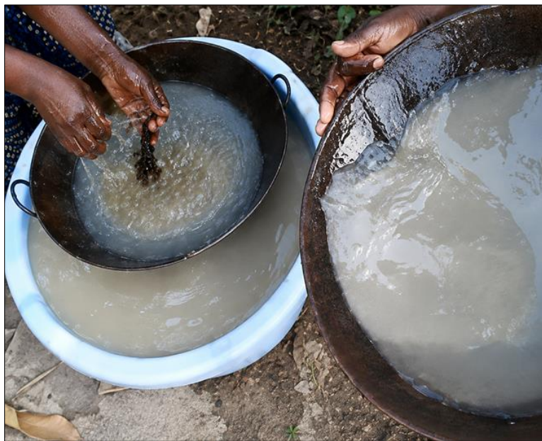
Fig 1: Washing recovered amalgam in shallow metal pans, a routine step that precedes the burning-off of mercury to isolate the gold sponge. (Researchers Fieldwork, 2026)
