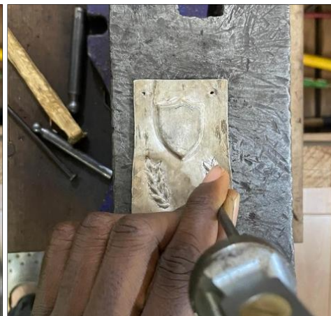
Fig 11: Chasing and repousse of leaf
