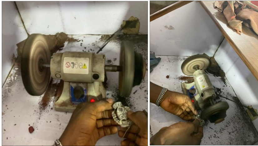
Fig 12: Using the tripoli to remove scratches Fig 13: Buffing for a glossy finish
