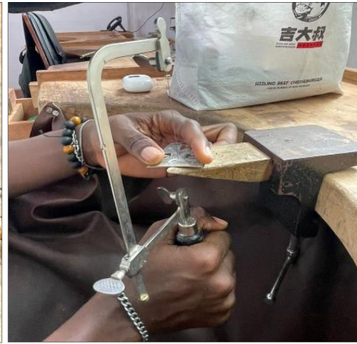
Fig 9: Piercing of letterings
